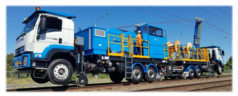
Manco Rail Road Rail Vehicle (RRV) for overhead line deployment, tensioning, and retrieval consisting of two interlocked 350HP cab/chassis vehicles connected via drawbar with fully interfaced engine, brake, and electronic controls
